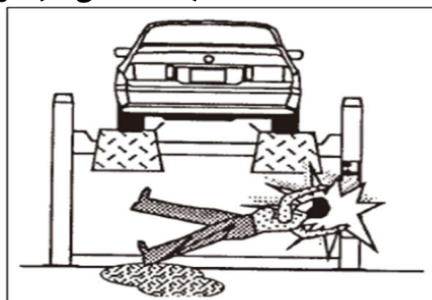
Figure 35 - Slip and fall risk
